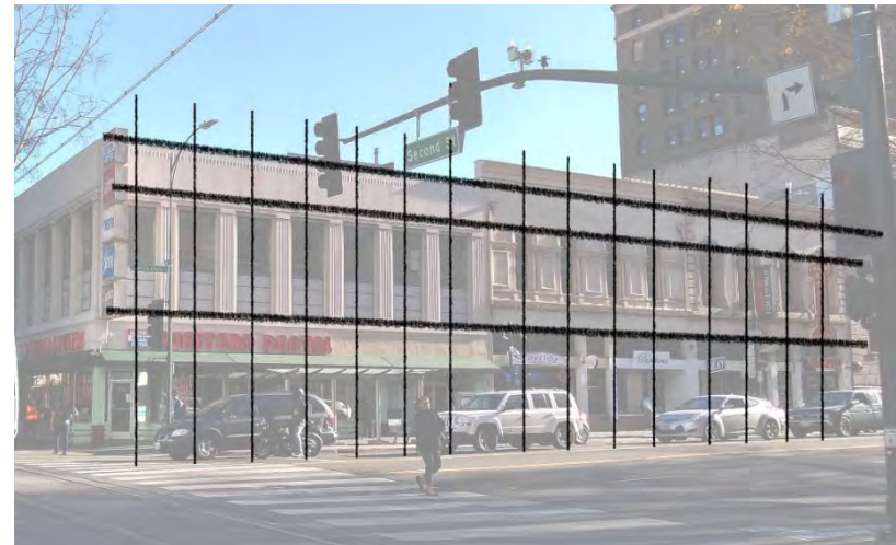
Use adjacent buildings as guides for floor heights and organization on new construction (Source: ESA)
