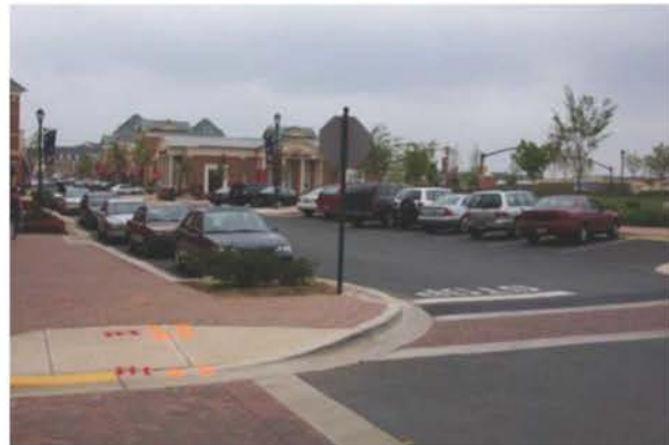
King Farm, a New Town in Rockville, Maryland, utilizes on-street parking to accommodate required parking spaces and alleviate the need for parking lots and structures. This street uses both parallel parking and angled parking.
